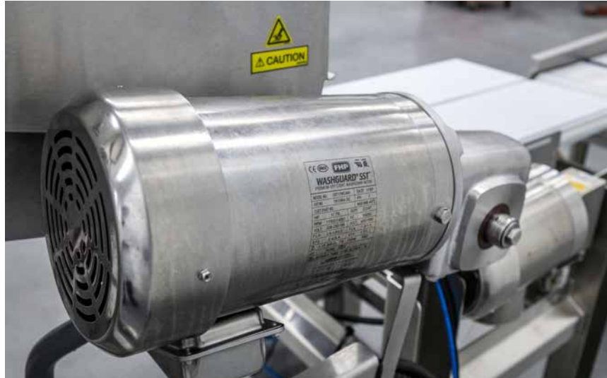
(Top) Close-up of the Leeson SST motor from Regal Beloit used to power the takeaway conveyor transporting chicken pieces from the Eagle X-Ray inspection system down the line for packing.
