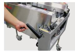
Tool-less case size changes are simple and quick with change points accessible from both operational sides of the machine.
