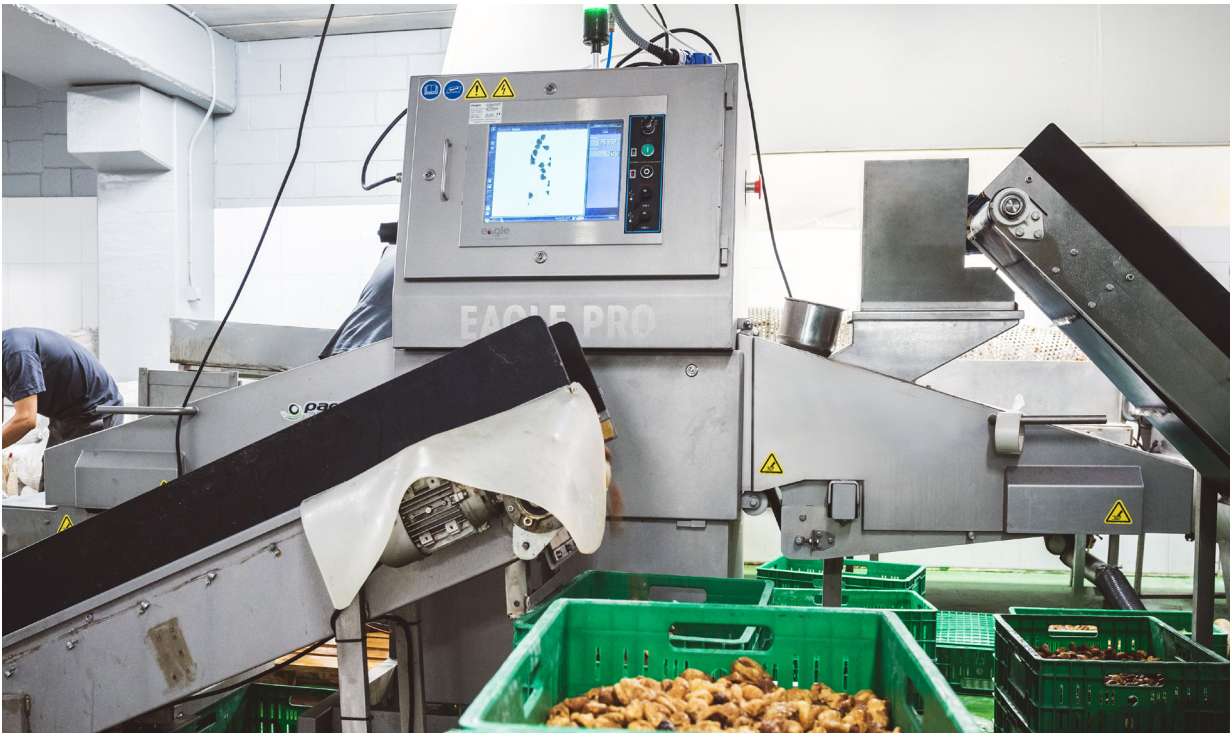
Eagle™ Bulk 415 PRO was installed by adapting the conveyor from the scalding system into the x-ray machine.
